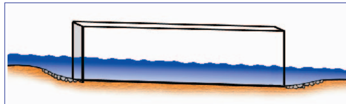
Fig. 2. Over-sized box culvert permanently backwatered
